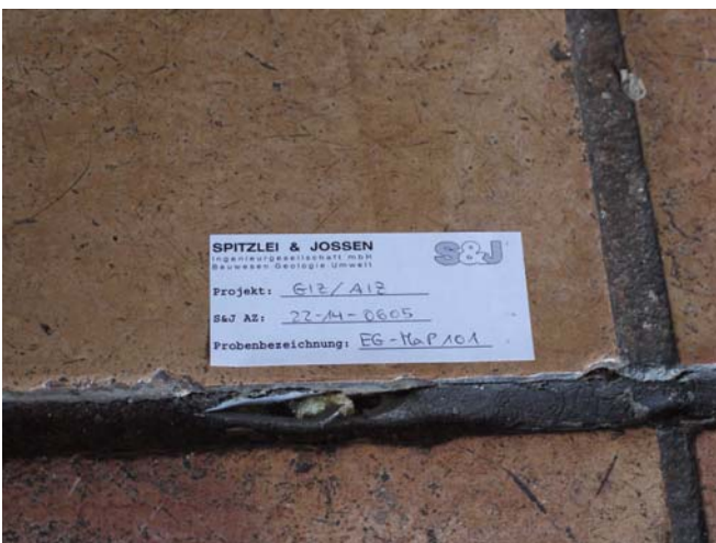
Foyer/Bar, Probe EG-MaP 101 (PCB)
